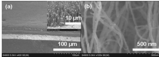
FIG. 2. SEM images of a CNT array synthesized on a pure Cu sheet. (a) Cross-section view of the vertically oriented and dense CNT array. The array height is estimated to be approximately 20  $\mu\text{m}$ ; the inset shows the CNT array grown on a 1 cm tall Cu bar from previous work (Ref. 15). (b) An image with higher magnification showing individual CNTs. The CNT diameters range from 15 to 60 nm.
