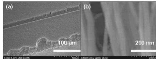
FIG. 1. SEM images of a CNT array synthesized on a Si substrate. (a) A  $30^\circ$ -tilted plane, top view of the vertically oriented and dense CNT array. The array height is estimated to be  $15 \mu\text{m}$ . The CNT array has a part across the top of the image that helps illustrate the uniformity of growth. (b) An image with higher magnification showing individual CNTs. CNT diameters range from 15 to 60 nm.
