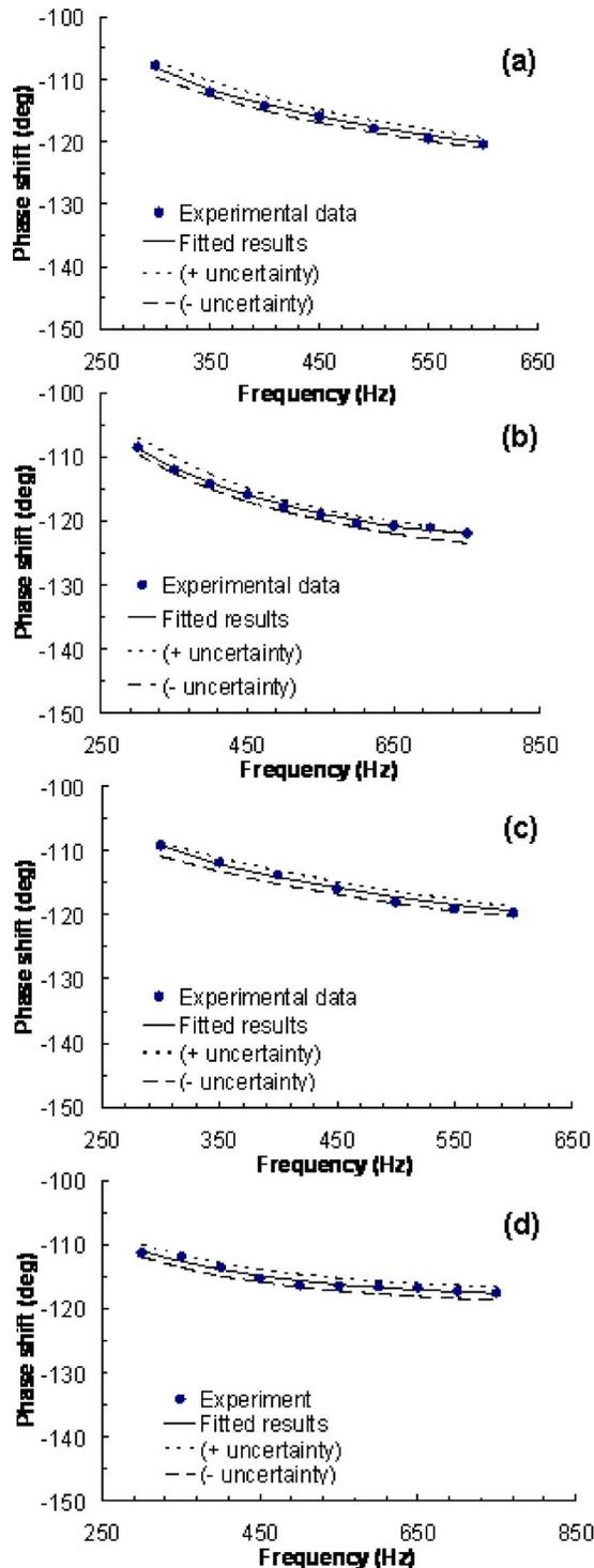
FIG. 6. (Color online) Phase shift as a function of modulation frequency for CNT interfaces with an applied contact pressure of 0.241 MPa. The mean-square deviation of all fits is approximately  $0.3^\circ$  in phase shift. (a) Lumped one-sided interface fitting results. (b) Resolved one-sided interface fitting results. (c) Lumped two-sided interface fitting results. (d) Resolved two-sided interface fitting results. The two-sided fitting data are typical of measurements at each pressure.
