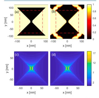
**Figure 5.** Density distribution of the original bowtie structure (a) and the final design structure (b) overlaid with surface *S* marked by red dashed line and their respective electric fields distribution on surface *S* (c, d). The electric fields distribution is normalized by incident wave intensity.
