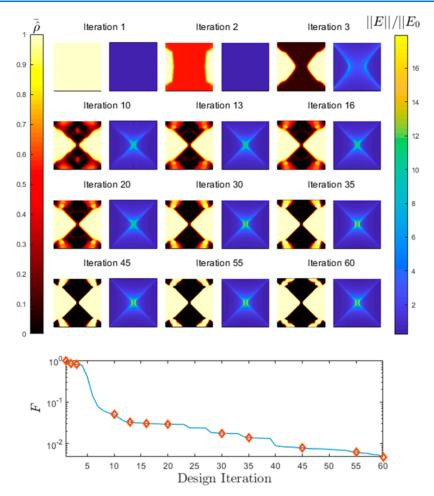
**Figure 6.** Distributions of the projected density  $\overline{\rho}^{i}$  (left) and the field magnitude (right) in some intermediate steps showing the evolution of the density. Each iteration is marked with a diamond in the objective function graph at the bottom. The objective function is normalized so that it is evaluated as 1 in the first iteration.
