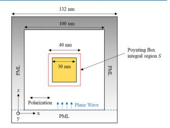
**Figure 2.** Layout for the example. A block of size  $30 \times 30 \times 30 \mod^3$  is seated in an open region with its axis aligned with coordinates. An incident plane wave travels in the  $z^+$  direction. PMLs of eight-cell thickness are used to absorb any outgoing waves. The Poynting flux is integrated on the box surrounding the block.
