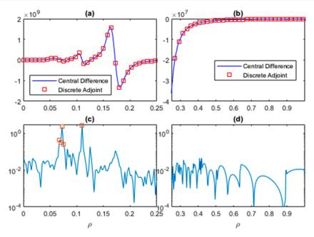
Figure 3. (a, b) Comparison of the central difference sensitivity and the discrete adjoint sensitivity. (c, d) Relative error of the discrete adjoint calculated by  $\delta(\rho) = |f'_{\text{discrete adjoint}} - f'_{\text{central difference}}|/|f'_{\text{central difference}}|$ ; points marked in squares are values larger than 0.2.
