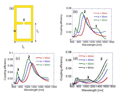
Fig. 7. (a) Schematic of the double loop SRR with the relevant dimensions, (b) Coupling efficiency into the recording medium versus wavelength for different values of w and the arm length  $l_x$ . (b)  $l_x = 120$  nm, (c)  $l_x = 150$  nm and (d)  $l_x = 250$  nm.
