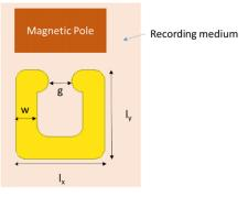
Fig. 3. Schematic of a single loop SRR showing the relevant parameters and the placement of the magnetic pole and the recording medium.
