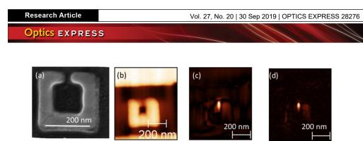
Fig. 11. s-NSOM results of SRR structure. (a) SEM image of an SRR structure, (b) AFM topography, (c) 2<sup>nd</sup> harmonic image of s-NSOM signal, and (d) 3<sup>rd</sup> harmonic image of s-NSOM signal.
