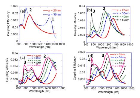
Fig. 6. Coupling efficiency into the recording medium versus wavelength for different values of w and the arm length  $l_x$ . (a)  $l_x = 90$  nm, (b)  $l_x = 150$  nm, (c)  $l_x = 200$  nm and (d)  $l_x = 250$  nm.
