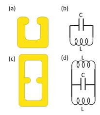
Fig. 1. (a) Schematic of a single loop split ring resonator nanostructure, (b) its equivalent LC circuit, (c) double loop SRR and (d) its equivalent LC circuit.
