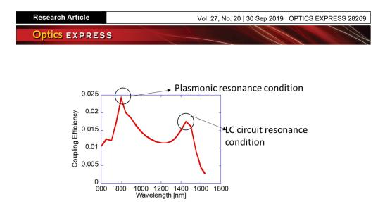
Fig. 4. Coupling efficiency versus wavelength for a single loop SRR.
