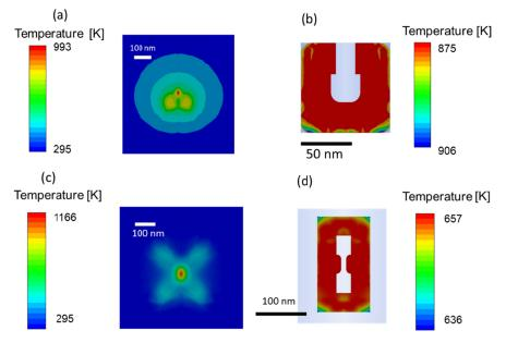
Fig. 9. For a single loop SRR, temperature plots of (a) recording medium at the end of 1 ns and (b) the NFT at steady state. For a double loop SRR, temperature plots of (c) recording medium at the end of 1 ns and (d) the NFT at steady state.
