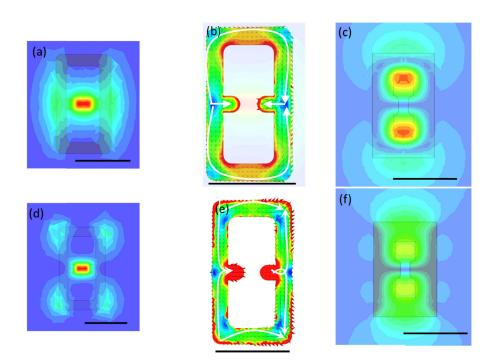
Fig. 8. (a) Electric field profile at the recording medium corresponding to mode (1), (b) Surface current density of the NFT for mode (1), (c) Out-of-plane magnetic field for mode (1), (d) Electric field profile at the recording medium corresponding to mode (2), (e) Surface current density at the surface of the NFT for mode (2) and (f) Out-of-plane magnetic field for mode (2). (Modes (1) and (2) denote the resonance peaks as seen in Fig. 7(b)). Scale bar in these figures is 150 nm.
