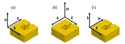
Fig. 2. Possible orientations of the propagation vector of the incident light and the electric and magnetic field polarizations to excite resonance mode in the SRR structure. (a) The magnetic field is pointed out-of the plane with the electric field pointed parallel to the gap, (b) The magnetic field is pointed out of the plane with the electric field pointed across the gap and (c) The propagation vector is pointed out of the plane with the electric field pointed across the gap.
