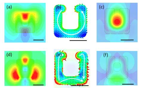
Fig. 5. (a) Electric field profile at the recording medium at 1550 nm, (b) Current density at the surface of the NFT at 1550 nm, (c) Out-of-plane magnetic field at the recording medium at 1550 nm. (d) Electric field profile at the recording medium at 800 nm, (e) Current density at the surface of the NFT at 800 nm and (f) Out-of-plane magnetic field at the recording medium at 800 nm. Scale bar in these figures is 50 nm.
