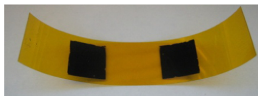
Figure 6. Picture showing the transfer of 1 \text{ cm} \times 1 \text{ cm} VACNT arrays to polyimide tape. The ease of transfer was aided by etching the nanotubes using an Ar–H 2 O flow rate of 80 sccm.
