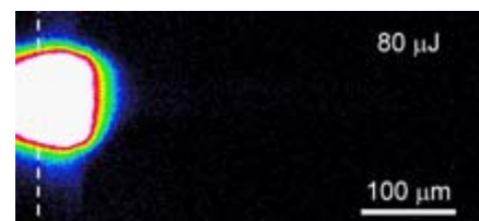
FIG. 5. (Color online) Experimental plasma radiation of single pulse focused on sample surface with 80 \mu\text{J}/\text{pulse} .
