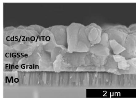
Fig. 4. SEM cross-section of champion device
