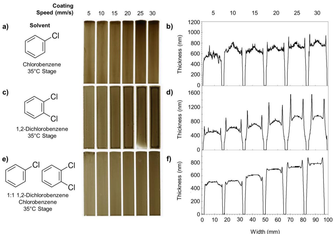
Fig. 1. Color scans and generated width profiles from CIGS nanoparticle inks with various solvents. a) Color scans of chlorobenzene ink films and b) their generated thickness profiles across the width. c) Color scans of 1,2-dichlorobenzene ink films and d) their generated thickness profiles across the width. e) Color scans of chlorobenzene/1,2-dichlorobenzene cosolvent ink films and f) their generated thickness profiles across the width.
