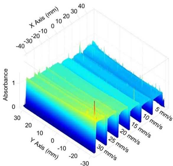
Fig. 2. 3D film reconstruction via absorbance scanning showing minimal "coffee ring" and increased width and length uniformity using the CB/DCB co-solvent
