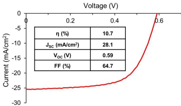
Fig. 5. J-V sweep for the champion device with a total area efficiency of 10.7%
