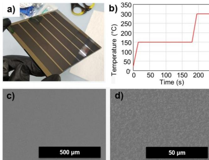
Fig. 3. a) An image of a molybdenum coated substrate with stripes of CIGS nanoparticles b) A representative annealing profile to prevent cracking c) / d) SEM micrographs of the nanoparticle film surfaces showing largely microcrack free films
