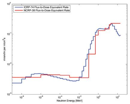
**Fig. 1:** Variation of neutron flux-induced dose versus neutron energy. Data from International Committee on Radiological Protection (ICRP) Publication 74, *Conversion Coefficients for Use in Radiological Protection against External Radiation* (1996), and National Council on Radiation Protection and Measurements (NCRP) Report 38, *Protection against Neutron Radiation* (1971).
