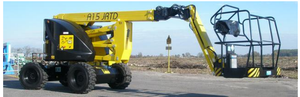
Fig 1a – prototype of the articulated boom lift
