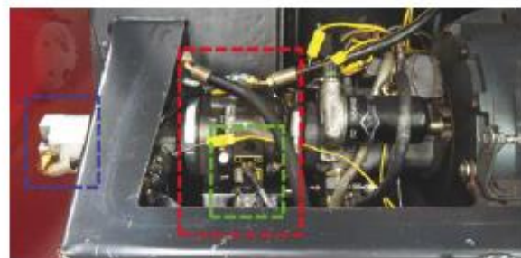
Figure 3. DC steering system hydraulic components: the steering pump is enclosed in the red dashed rectangle, the proportional control valve is enclosed in the green dashed rectangle, and the charge pump is enclosed in the blue dashed rectangle.
