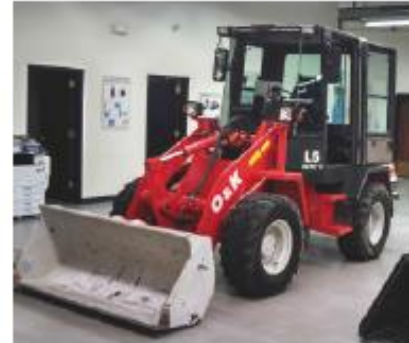
Prototype test vehicle with DC steer-by-wire system.
