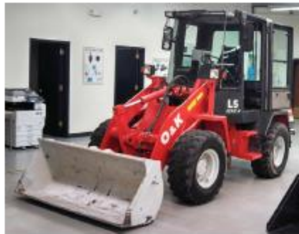
Figure 1 | Testing in the front loader shown indicates that a new technology known as pump-controlled steering exhibits superior fuel savings and productivity compared to standard hydraulic steering. (Courtesy of Purdue University)
