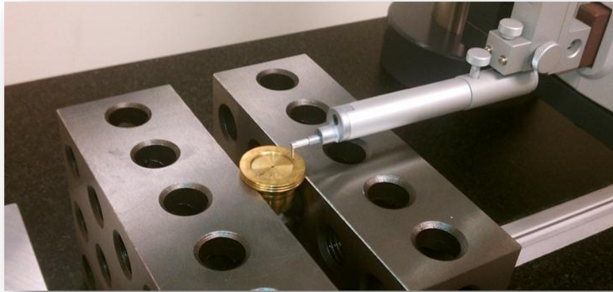
Figure 15: Measuring slipper wear using the Mitutoyo stylus profilometer
