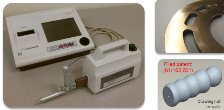
(Left) The Mitutoyo stylus surface profilometer. (Right Top) A manufactured waved valve plate. (Right Bottom) Exaggerated illustration of a micro-wave shaped piston.
