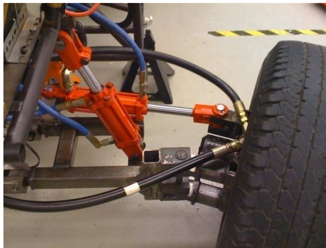
Hydraulic Pump Controlled Steering System
