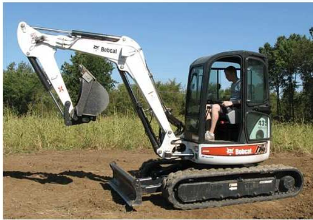
Small excavator used to test pump-controlled actuation, in which traditional flow-control valves are replaced by with variable displacement pumps.
