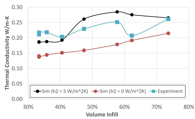
We hypothesized that the discrepancy between experiments and modeling was due to convection in the system. Simulations show that including convection increases the apparent thermal conductivity. There are still some variations between experimental and modeling results.
