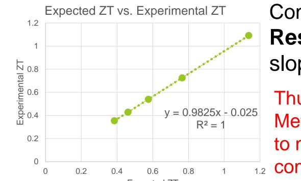
Comparison of ZT for materials with different k<sub>TF</sub> Result: the relationship is nearly linear with a slope ~1
