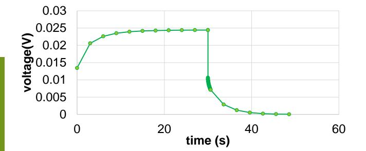
The voltage difference reaches the steady state with heat loss from the side walls. Although the times need to reach steady are different, all of them are less than 30s. Heat losses from the sides of the sample impact the accuracy of the measurements.
