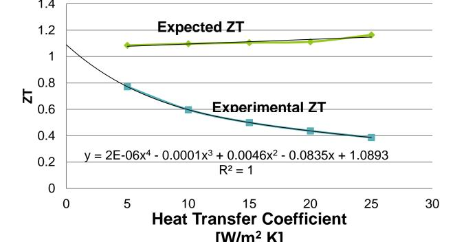
For the baseline case, the *ZT* using the extrapolation method reasonably matches the expected ZT input into the simulations. For cases where the Seebeck coefficient and electrical conductivity are changed, there is increased error in the extracted ZT (4 - 12 %).
