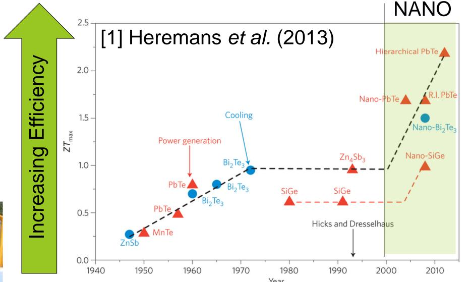
Nanostructuring improves the efficiency of thermoelectric materials by decoupling thermal and electrical transport.
