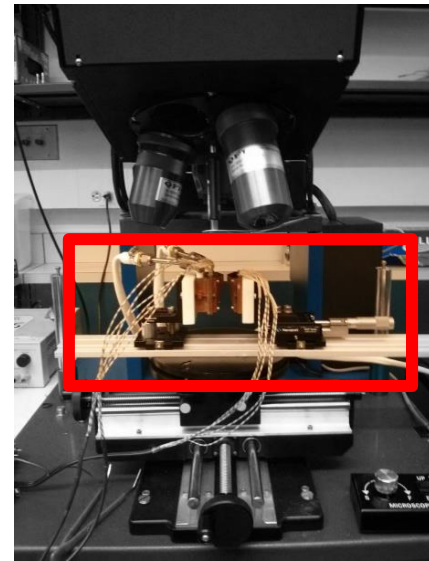
Figure 2. Miniature IR thermal conductivity measurement rig mounted on IR microscope stage. The components of thermal conductivity rig (in color and enclosed by red outline) are shown in Figure 1.
