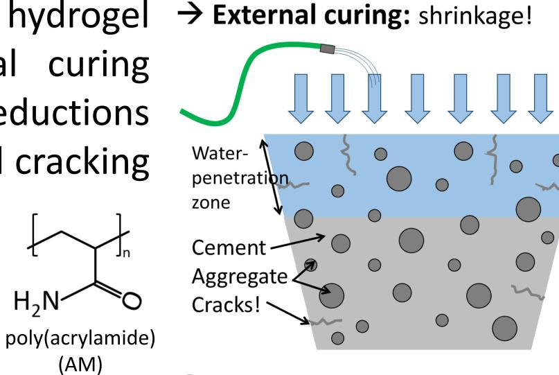
$\rightarrow$  Internal curing with gels: increased strength and durability!
