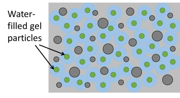
Despite voids remaining from deswollen hydrogels, mortar strength increased at 28 days, implying more complete curing and less microcracking from shrinkage:
