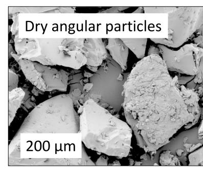
Hydrogel particle chemistry, shape, and size are controlled through different synthesis methods. Swelling behavior is strongly dependent on hydrogel chemistry (AA:AM).
