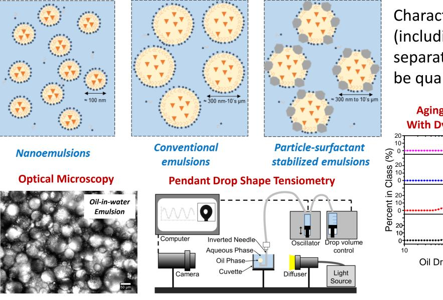
Characteristics which govern emulsion stability (including droplet size distribution, phase separation resistance, and interfacial elasticity) can be quantified using several techniques:
