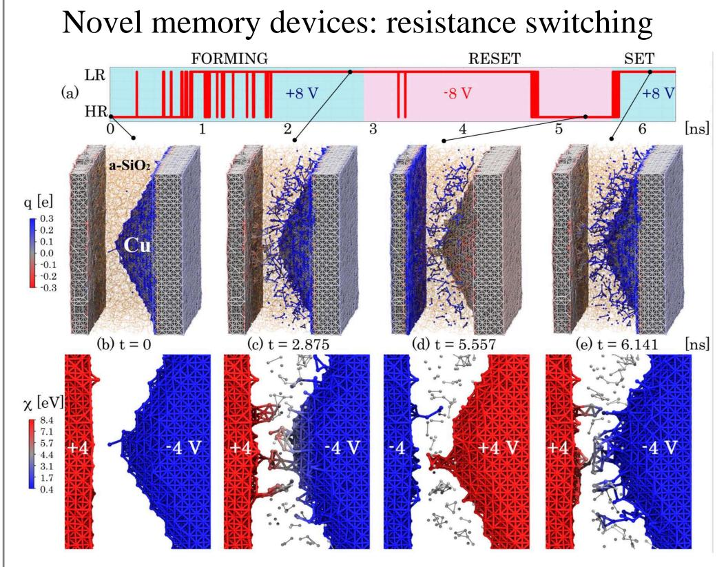
• Modeling the operation of an electrochemical electro-metallization cell • Uncover mechanisms behind ultra-fast switching
