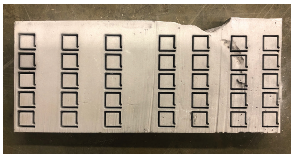
Aluminum ingot sectioned and cut into small cubes for optical and electron microscopy analysis.
