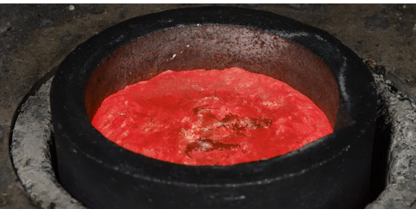
Molten aluminum alloy waiting to be cast into an ingot.
