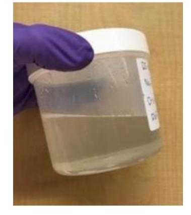
The polymer solution was poured polystyrene container coated with an organic mold release. The solution dried for 24 hours at room temperature on a flat surface with a cover to block dust (left).
