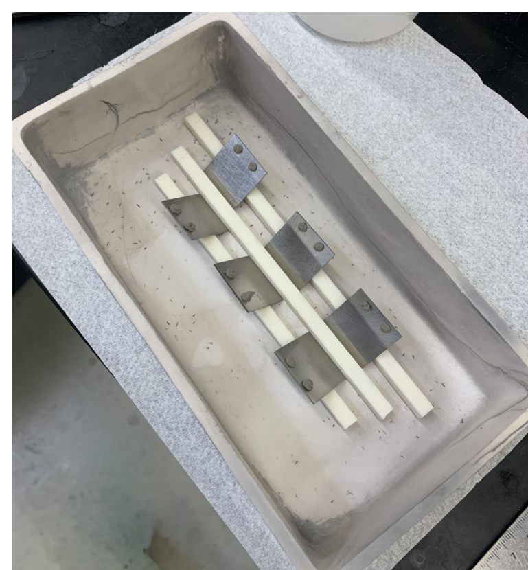
Figure 5: 40° braze setup pre-braze.
