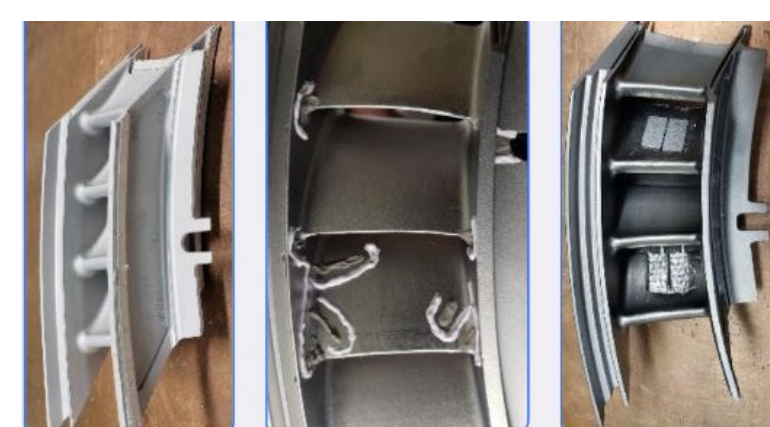
Figure 1: Examples of braze application on a turbine vane. From left to right: dimensional restoration, crack repair, feature replacement
