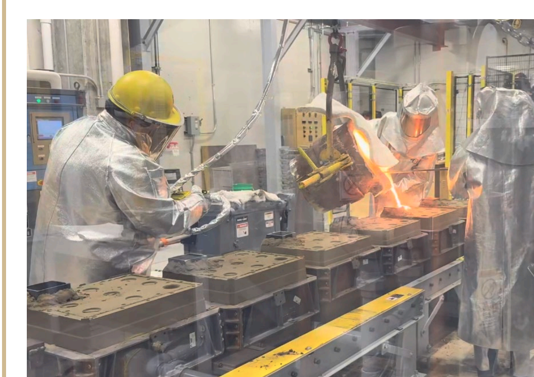
Figure 7. SiMo 5-1 DI pour in the SMART Foundry completed with MET.
