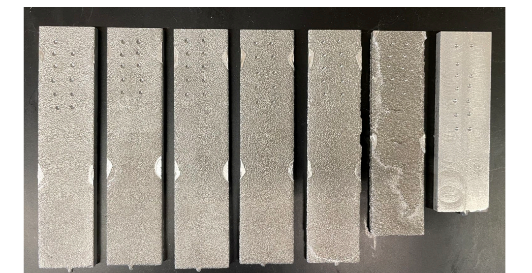
Nitrogen Cold Sprayed samples with Rockwell Hardness indents on post-peen surface
