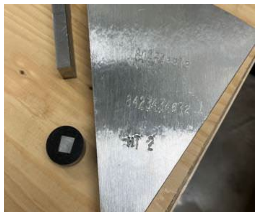
Figure 3. Section of 22" diameter Haynes® 242® ingot.
