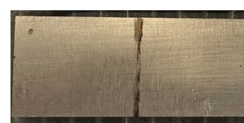
Typical developed wear groove.
