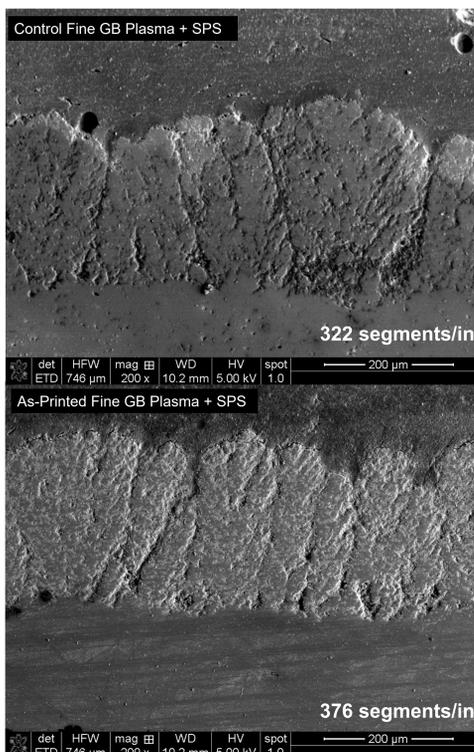
Figure 7: SEM imaging of sample cross-sections, consisting of an Inconel substrate, a plasma sprayed MCrAlY bondcoat, and an EBC top coat. The columnar microstructure of the SPS TBC is apparent.
