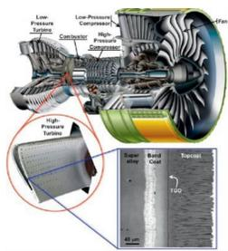
Figure 1: Gas turbine engine diagram including a schematic of the metal alloy, bondcoat, and top coat layers [1].
