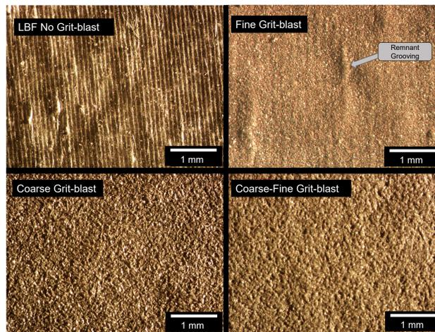
Figure 5: Stereoscope micrographs of surface of uncoated samples. As-printed and fine grit-blasted samples show a ridging effect. Coarse and coarse-fine grit-blasted samples show no remnant ridging effect.
