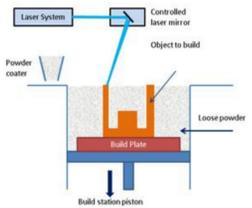
Figure 2: Diagram of the LBF process, illustrating the production of an AM part [2].
