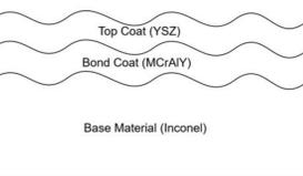
Figure 3: Illustration of changes to the AM surface affecting the bond and top coats on top of it.
