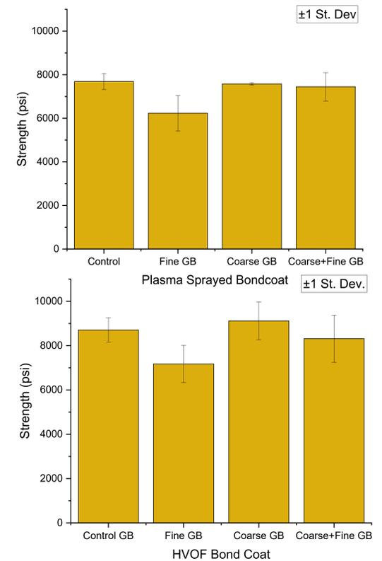
Figure 8: Results from bond cap (ASTM-C633) testing (n=3) for each surface condition, coated with both a bondcoat and top coat. In all cases failure occurred within the top coat. For both samples with HVOF and plasma sprayed bond coats on LBF substrates, standard fine grit-blast showed a debit in bond strength when compared to the control samples. That debit could be recovered by implementing a coarse grit blast, with or without a fine grit-blast following.
