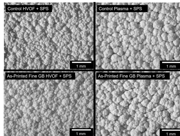
Figure 6: Stereoscope micrographs of samples coated with TBCs for HVOF bondcoats on left, and plasma sprayed bondcoats on the right. Top images show the morphology of the TBCs on control samples, while bottom images show equivalent coatings on the fine grit-blast LBF substrates. No clear difference observed as function of LBF ridging effect.
