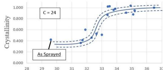
**Figure 3:** The LMP's and crystallinities of heat treated samples. Rapid crystallization occurs between LMP's of 75 and 76.
