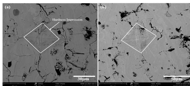
**Figure 2:** SEM Micrographs of the (a) as-deposited and (b) 20hr heat treated samples showing the hardness impression.
