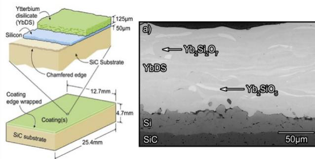
**Figure 1:** Diagram of an EBC bonding to a SiC/SiC substrate and the biphasic splat microstructure of the coating [1].
