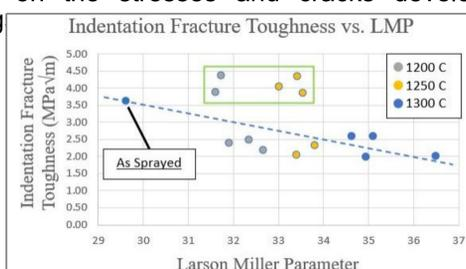
**Figure 5:** Indentation fracture toughness displays negative correlation with the Larson Miller Parameter. Low crystallinity samples (green) had higher fracture toughness.
