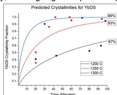
**Figure 4:** Substituting Avrami constants into the Avrami equation [3] estimates a phase's crystallinity after a heat treatment.
