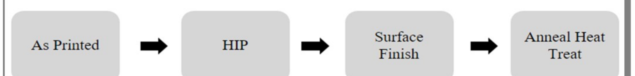
Figure 7: Recommended sequence of post-processing steps to obtain the desired final hardness and surface roughness.
