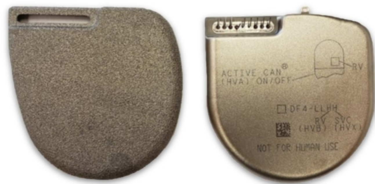
Figure 1: Image of Ti-6V-4Al shields used by Medtronic. On the left is a shield created through SLM, and on the right is the traditional deep drawn shield.
