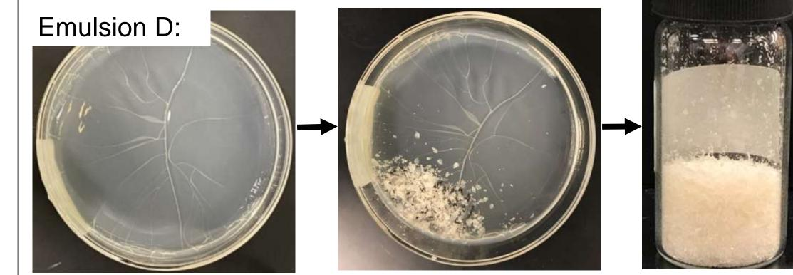
1 wt.% of flakes were added to room temperature DI water to observe dissolution of flakes:
