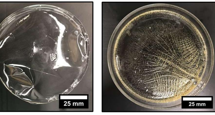
PVA (left) formed a stiff film that was unable to dissolve in water at room temperature while Capsul® (right) dissolved readily.
