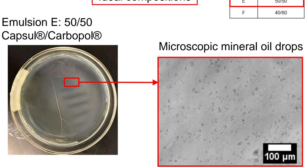
Optical microscopy showed successful encapsulation of mineral oil in a Capsul®-Carbopol® solution. Drops were evenly dispersed and had an average diameter of 1.14 µm. Casted film was continuous and dry to the touch, suggesting no oil loss.
