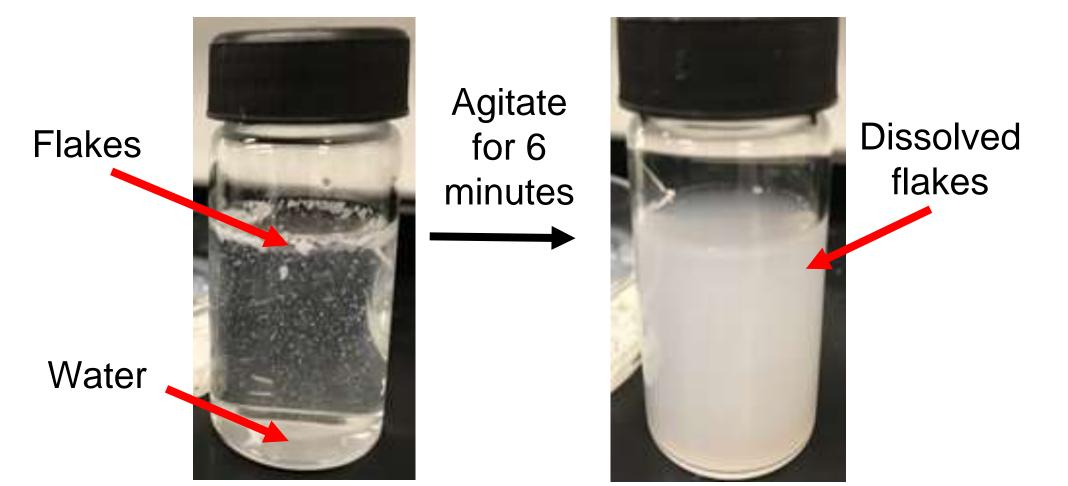
1 wt.% of flakes was successfully dissolved in room temperature DI water. Flakes also dissolved readily with water and shear against the palms.
