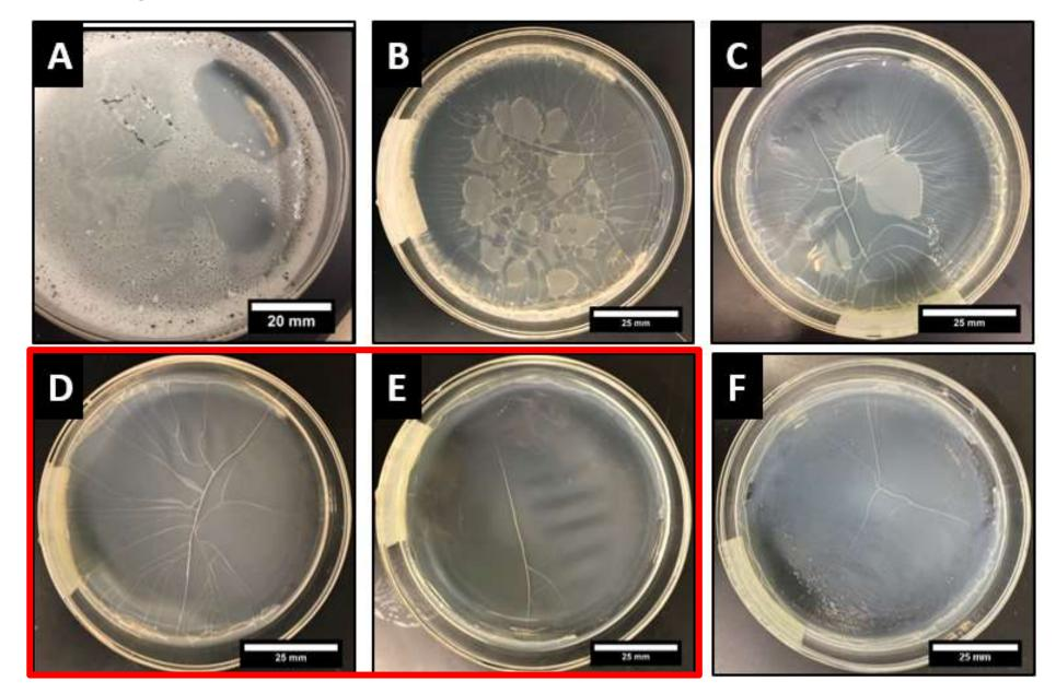
Capsul® and Carbopol® concentrations Capsul/Carbopol were varied but the ratio of mineral oil Emulsion Solutions [%/%] to aqueous solution was held constant at 1:4 oil to aqueous phase.
