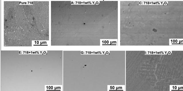
The SEM imaged revealed that after adding  $\text{Y}_2\text{O}_3$  no significant cracking was introduced to the system. Cellular structure was also observed in these samples.
