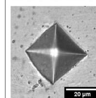
An indentation (right) on the surface of a cube sample describes the hardness of the material. A greater average diagonal length is indicative of a softer material. The microhardness is typically three times that of the flow stress, which is depicted in the table below
