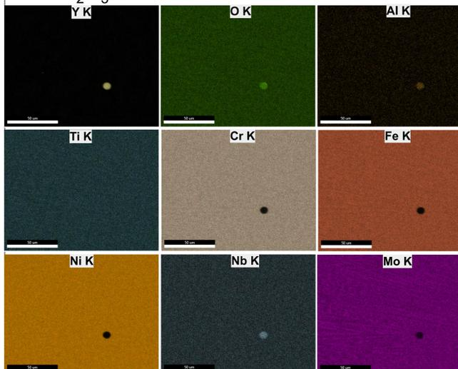
The EDS analysis confirmed the presence of the  $\text{Y}_2\text{O}_3$ , indicating that  $\text{Y}_2\text{O}_3$  particles can survive the high processing temperature.
