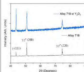
There were no drastic peak shifts when  $\text{Y}_2\text{O}_3$  particles were added to the Alloy 718 matrix. The variation of peak intensity indicated the texture variation.
