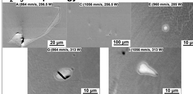
The morphology of the oxide particles depends on the printing parameters. The printing parameter E (960 mm/s, 285 W) leads to the smallest and spherical oxide particles. Whereas, agglomeration of yttria occurs when applying other printing parameters.
