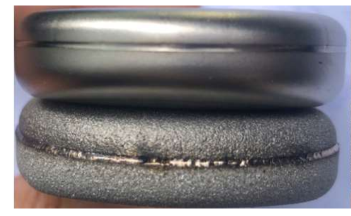
AM shield vs. deep drawn Rough AM shield (bottom) has poor weld seal quality
