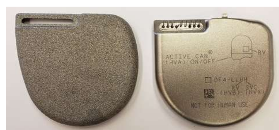
AM shield vs. deep drawn Rough AM shield (bottom) has poor weld seal quality
