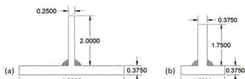
Figure 2: Rendering schematics of our sample dimensions, (a) ASTM A709 and (b) AISI 1018
