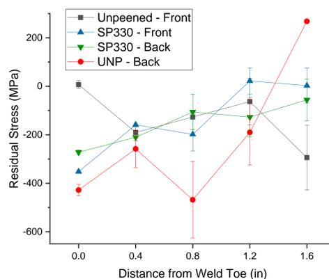
Figure 5: Topographical profile of residual stress for A709.
