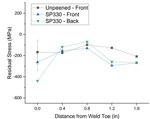
Figure 6: Topographical profile of residual stress for 1018.
