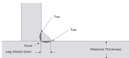
Figure 1: Schematic of a T-joint sample showing the location of weld toes.
