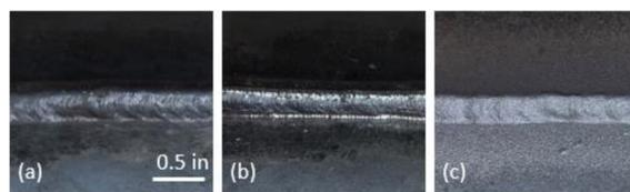
Figure 3: Close-up images of the A709 steel; (a) control, (b) UNP and (c) SP
