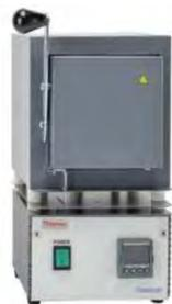
Figure 4. A FB1400 Thermo Scientific Thermolyne furnace used to heat treat samples at different temperatures for 9 weeks.
