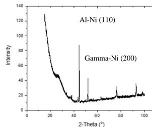
Figure 7. A representative XRD spectra is seen for the PM400 samples. This spectra was constant with all samples including the heat treated ones. The major peaks are indexed as seen.
