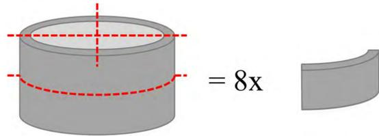
Figure 3. Example bushing with red dotted lines indicating where sectioning occurred. This shows how 8 specimen we pulled from the sample.
