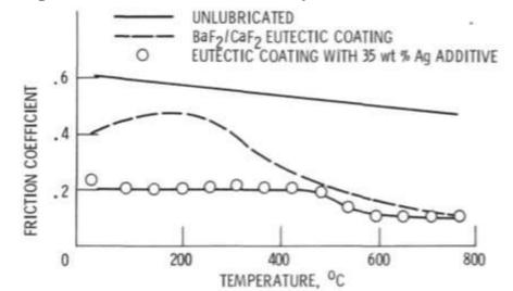
Figure 10. Friction coefficient vs temperature for surfaces with and without solid lubricant coating [2].
