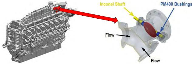
Figure 1. Caterpillar G3616 A4, a natural gas fueled engine with the wastegate valve highlighted in red. The wastegate assembly is magnified on the right with the components marked.
