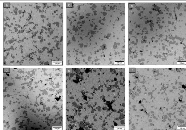
Figure 5. SEM imaging of samples (a) 34.1, (b) 34.2, (c) 34.3, (d) 34.4, (e) 34.6, and (f) field sample B1. Samples 34.1-34.6 were heat-treated at 500°C for 12, 24, 48, 96, and 500 hours, respectively.
