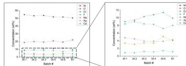
Figure 9. Experimental EDS data for 500°C tempered PM400 samples 34.1-34.6 and field sample B1 for elements Ni, O, Cr, F, Mo, Ag, and Ca.
