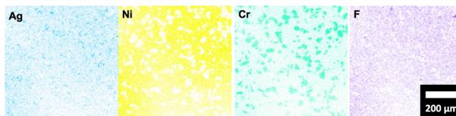
Figure 8. EDS color maps are seen outlining the silver, nickel, chromium, and fluorine present in the system. The sample shown was heat treated for 12 hours at 500 C.
