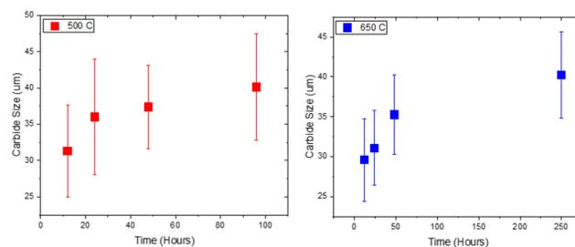
Figure 6. The charts show the average oxide size across different heat treatment times for a given temperature (500 C on left and 650 C on right). This graph represents the precipitation of the oxides on the system.
