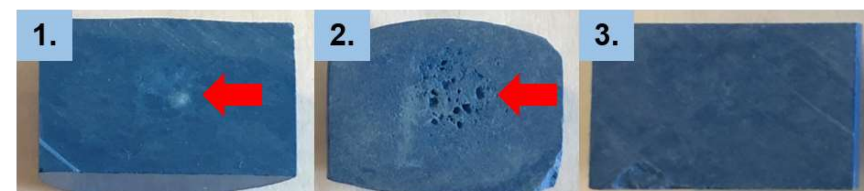
Figure 5: Cross-section photographs of DAP specimens #1, 2 and 3 after ethanol testing. Arrows indicate discoloration and/or pores in uncured regions. Each sample is 1.25 inches in diameter (0.0318 m).
