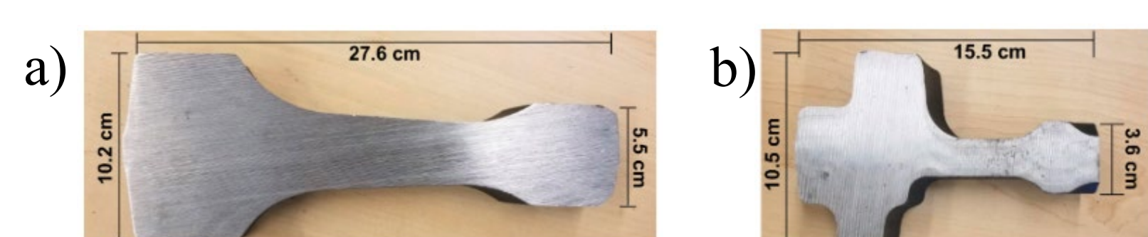
Figure 4: a) The large and b) small turbine wheel radial cross-sections
