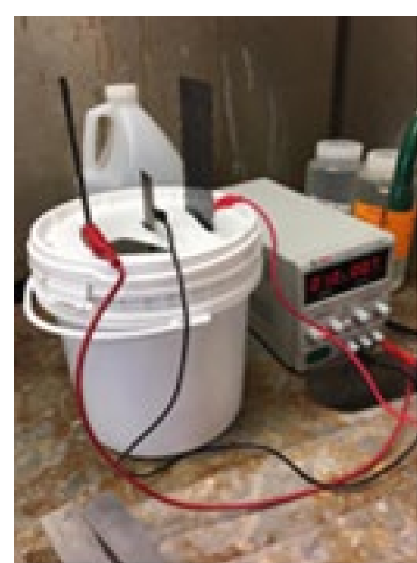
Figure 2: Hydrogen charging apparatus used for this project
