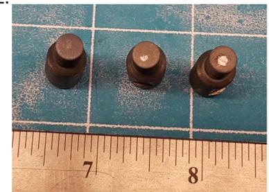
**Figure 7:** Wear scars (from right to left) of pins run under the following conditions: lubricated 30 min. test for P1, lubricated 30 min. test for P6, and non-lubricated 20 min. test for P6.
