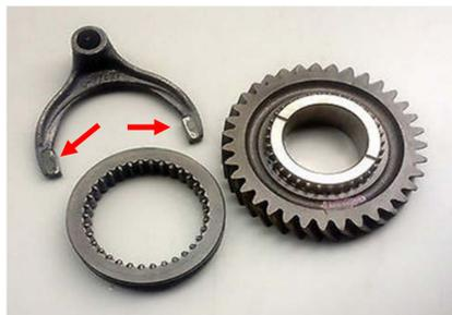
**Figure 1:** Shifter fork (top left) with synchronizer and gear. Arrows indicate wear surfaces that receive the spray coating.
