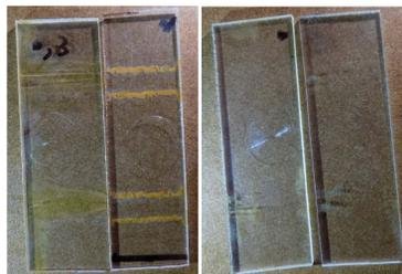
Samples after exposure to 2-(2-butoxyethoxy)ethanol (left) and Polyalkylen derivate (right) baths for five days under strain.
