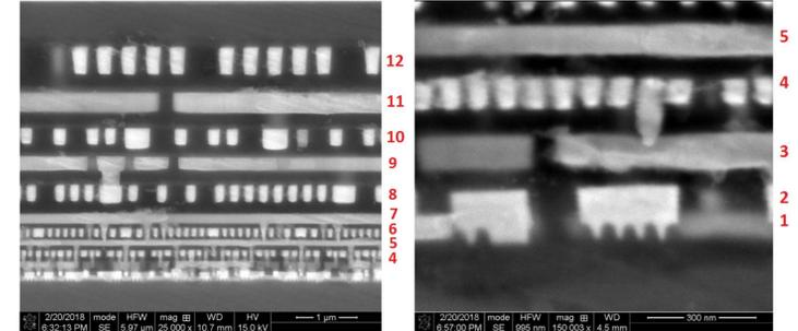
A SEM image of the Cu interconnects before thermal cycling is shown on the left. An enlarged SEM image of the metal lines representing the thinnest layers is shown on the right.
