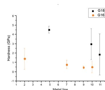
The graph to the left shows the hardness data for the Cu interconnects for G16 and G18 CPU samples. Depth refers to the contact depth from the starting point. The metal line number correlates to the labeled metal lines in the SEM images above.
