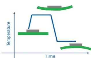
With long term operation, these stresses may lead to a failure after multiple temperature cycles. Temperature cycle testing is a method of acceleration testing for products that experience variation in temperature under a daily use basis. Since this experiment is focused on the effect of the extended thermal cycling on the Cu interconnects, a Coffin-Manson model was used to calculate the low cycle fatigue specifications to use in testing.
