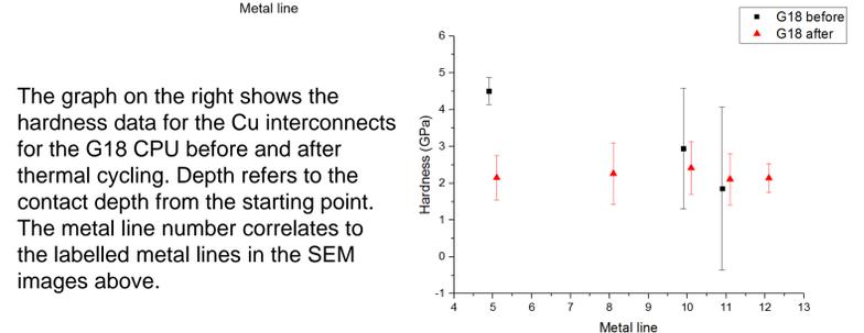
The graph on the right shows the hardness data for the Cu interconnects for the G18 CPU before and after thermal cycling. Depth refers to the contact depth from the starting point. The metal line number correlates to the labeled metal lines in the SEM images above.
