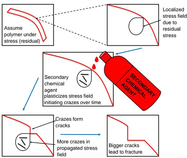
Figure 1: Mechanism of failure through Environmental Stress Cracking.
