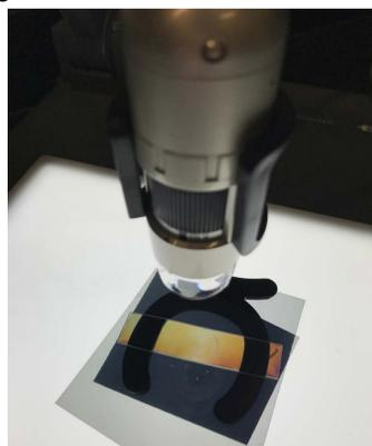
Figure 3: Imaging of tested samples using Dino-lite microscope and cross-polarizers.
