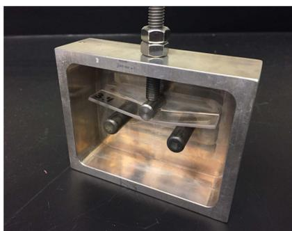
Figure 2: Jig with sample under stress ready to be submerged in coolant.
