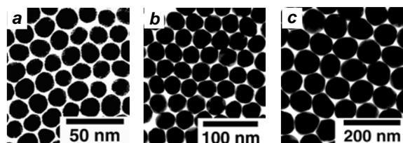
**Figure 2.** TEM images of Au nanoparticle films transferred onto Formvar-coated Cu grids (Philips EM-400, 80-100 keV). Unit particle sizes: (a)  $16 \pm 3$  nm; (b)  $34 \pm 2$  nm; (c)  $87 \pm 7$  nm.
