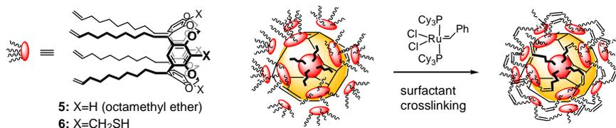
**Figure 9.** Gold nanoparticles encaged in a crosslinked resorcinarene shell.
