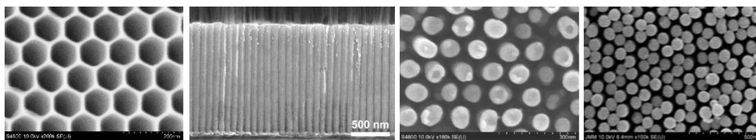
**Figure 6.** FE-SEM images of 2D Au nanorod arrays. (a) nanoporous  $\text{Al}_2\text{O}_3$  template; (b) cross-section of 2D nanorod array ( $h = 1.396 \pm 0.007 \mu\text{m}$ ); (c) 2D array of nanorod tips; (d) free-standing 2D nanorod array.
