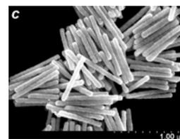
**Figure 11.** Au nanorods (750 nm) prepared by templated electrodeposition in nanoporous Al<sub>2</sub>O<sub>3</sub>.
