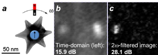
**Figure 18.** (a) Gyromagnetic Au nanostar with Fe<sub>3</sub>O<sub>4</sub> core. (b) Time-averaged image of magnetically active NST (left) inside KB cell under low-lighting conditions, next to brighter but static scatterer. (c) Gyromagnetic 2 $\omega$ -filtered image. Images are 8 x 8  $\mu$ m.
