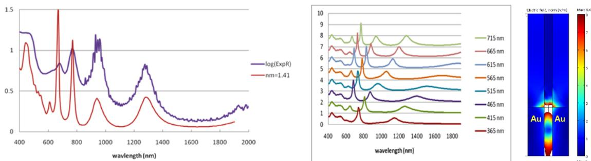
**Figure 7.** (a) Experimental and simulated absorbance–reflectance spectra from Au nanorod arrays on a 50-nm Au baseplate. (b) Collective plasmon resonances as a function of nanorod height ( $d=75$  nm; 105 nm spacing). (c) Local field factors ( $E/E_0$ ) between gold nanorods near tips (white region is offscale).
