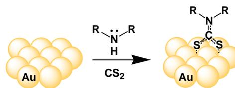
**Figure 10.** Assembly of dithiocarbamates on Au.
