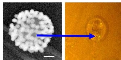
**Figure 8.** *Left*, 40/350-nm Au/SiO<sub>2</sub> superparticle ensemble (scale bar = 100 nm). *Right*, tSA201 cell subjected to nanoprobe implantation.
