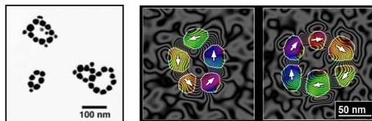
**Figure 3.** *Left*, ferromagnetic Co nanoparticles self-assemble into “bracelets” when dispersed in toluene with resorcinarene **1**. *Right*, chiral FC states in Co nanorings with CCW and CW polarizations, as visualized by electron holography.
