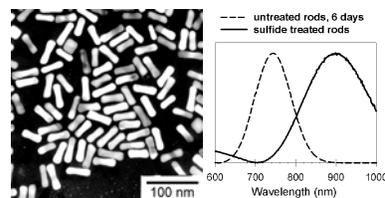
**Figure 12.** Au nanorods ( $L < 50$  nm) prepared by a seeded growth process and stabilized by sulfide quenching.
