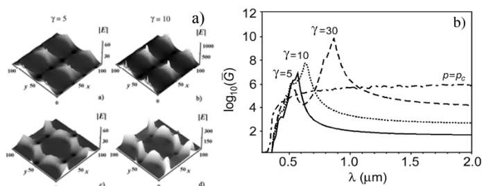
**Figure 5.** (a) Spatial distribution map of plasmon-generated fields from two metal nanoparticles at different interparticle spacings. (b) Average signal enhancements ( $G$ ) from 2D arrays of Au nanodisks as a function of  $\lambda_{\text{ex}}$  at fixed particle diameter–spacing ratios ( $\gamma = 5, 10,$  and  $30$ ). Enhancements from random metal–dielectric films at the percolation threshold ( $p = p_c$ ) are included for comparison.
