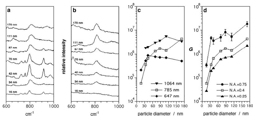
**Figure 4.** Tunable SERS activity from gold nanoparticle arrays. (a, b) Raman spectra obtained by excitation at 647 nm and 1064 nm; (c) signal enhancement factors ( $G$ ) as a function of periodic structure and excitation wavelength; (d)  $G$  as a function of numerical aperture (N.A.) at a fixed excitation wavelength (785 nm).
