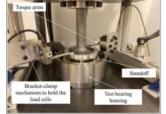
**Objective:** To experimentally examine the cage motion and ball-cage contact forces for an angular contact ball bearing (ACBB) operating under various load and speed combinations
