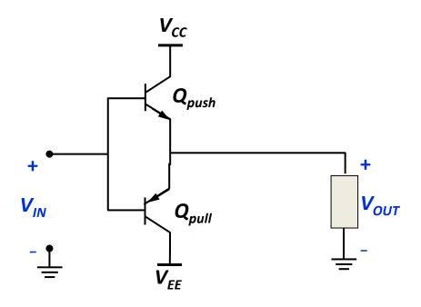
Push-Pull (class B) power (output) stage
