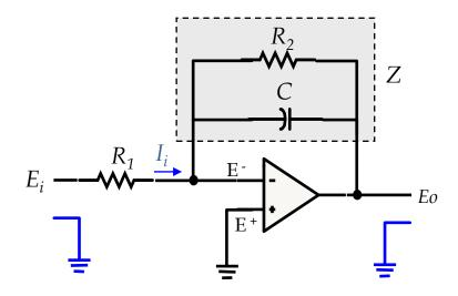
$$Z = \frac{1}{\frac{1}{R_2} + j\omega C} = \frac{R_2}{1 + j\omega R_2 C}$$
