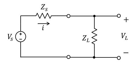
$$P_{L} = V_{L} i = \left(\frac{Z_{L}}{Z_{S} + Z_{L}} V_{S}\right) \left(\frac{V_{S}}{Z_{S} + Z_{L}}\right) = \frac{V_{S}^{2}}{\frac{Z_{S}^{2}}{Z_{L}} + 2 Z_{S} + Z_{L}}$$
