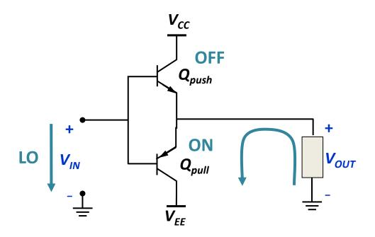
Push-Pull (class B) power (output) stage
