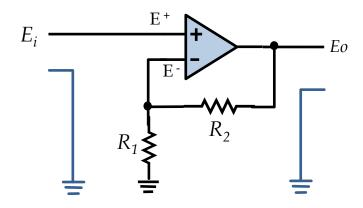
$$E_i = \left(\frac{R_1}{R_1 + R_2}\right) E_O \Rightarrow E_O = \left(\frac{R_1 + R_2}{R_1}\right) E_i$$
