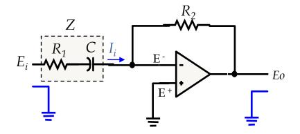
$$Z = R_1 + \frac{1}{j\omega C} = \frac{j\omega R_1 C + 1}{j\omega C}$$
