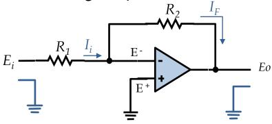
$$\frac{E_i - E^-}{R_1} = I_i = I_F = \frac{E^- - E_0}{R_2}$$
