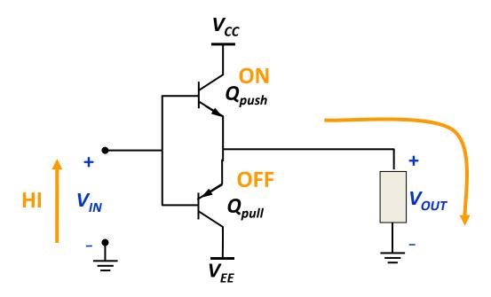
Push-Pull (class B) power (output) stage
