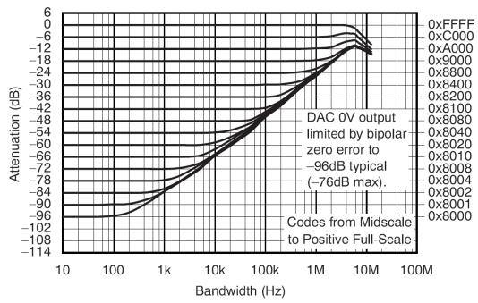
DAC8822: attenuation vs. reference multiplying bandwidth at various digital codes
