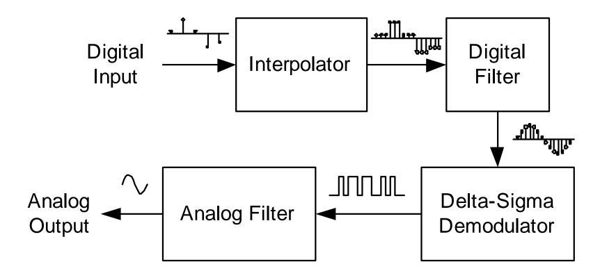
A Delta-Sigma-DAC is basically an DS-ADC operated in reverse direction: Oversampling of the digital input, digital filtering, demodulation, analog filtering. Predominantly used in Audio-DACs.
