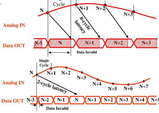
Huge delay -> Delta Sigma with multiple Fdata Delay from FIR with linear Phase (number of TAPS/2), e.g. 78 Fdata delay
