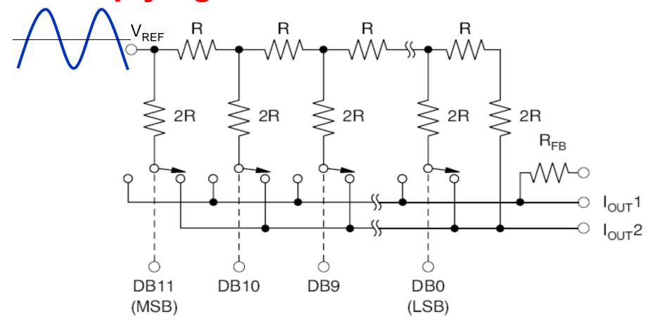
The above structure is essentially a R-2R-architecture. The "invisible" difference is , that  $V_{REF}$  can be an analog signal, i.e. an alternating signal, even crossing zero Volts.
