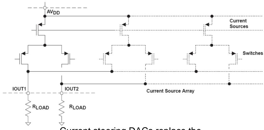
Current steering DACs replace the resistor arrays of R-2R-DACs with weighted current sources
