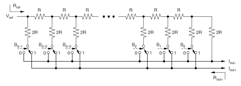
This classical approach delivers a current mode output. For voltage mode output, this structure is followed by an I/V converter
