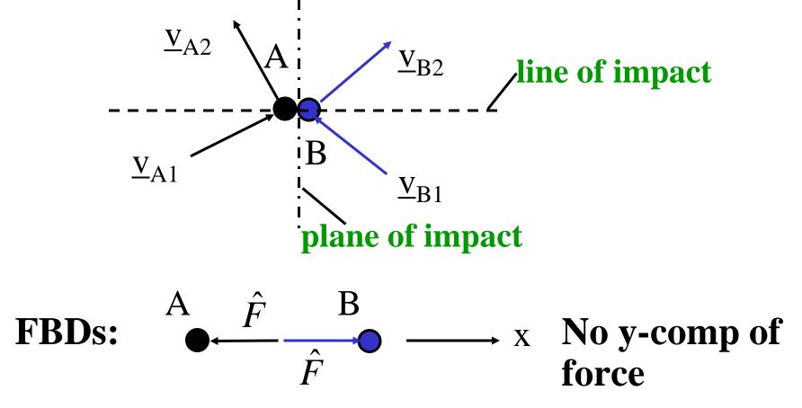
Let  $\underline{v}_A = v_{Ax}\underline{i} + v_{Ay}j$  and  $\underline{v}_B = v_{Bx}\underline{i} + v_{By}j$ be velocities;  $\underline{v}_{A1}, \underline{v}_{B1}$  before, and  $\underline{v}_{A2}, \underline{v}_{B2}$  after. The coefficient of restitution is then defined as: the ration of the relative velocity after impact to the relative velocity before impact, for velocities along the line of impact:
