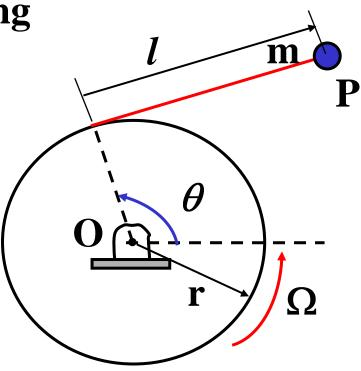
slip relative to the drum ; At t = 0,  $\ell(0) = 0$ ,  $\dot{\ell}(0) = r\Omega$ Find: Tension in the rope as a function of time.
