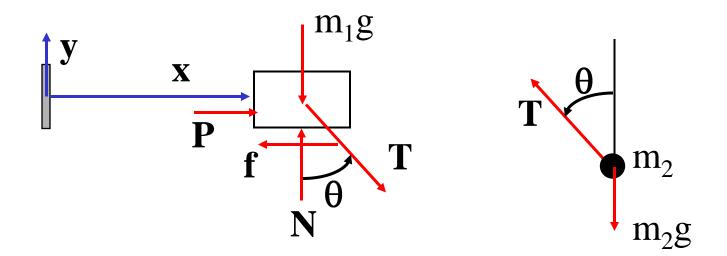
The positions of the two particles can now be defined:  $\underline{r}_1(t) = x(t)\underline{i}$  $\underline{r}_2(t) = \{x(t) + l\sin\theta\}\underline{i} - l\cos\theta\underline{j}$
