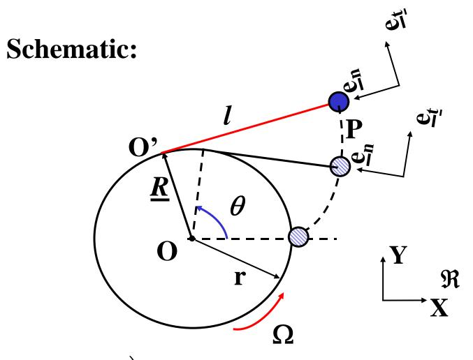
$(\underline{e}_t, \underline{e}_n, \underline{e}_b)$ - triad for moving coordinate system Let  $\underline{\omega}$  be angular velocity of the moving frame.
