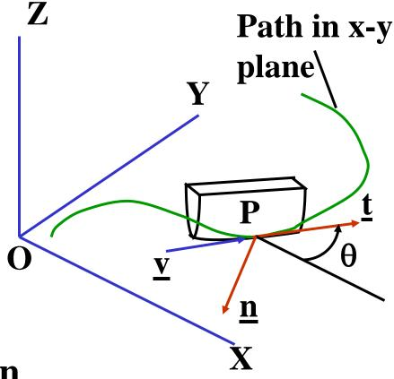
Let  $\underline{t}$  - tangent to the path,  $\underline{n}$  - normal to the path. Then  $\underline{v} \cdot \underline{n} = 0$  for the skate, or  $(\dot{x}\underline{i} + \dot{y}\underline{j}) \cdot (-\cos\theta\underline{j} + \sin\theta\underline{i}) = 0$
