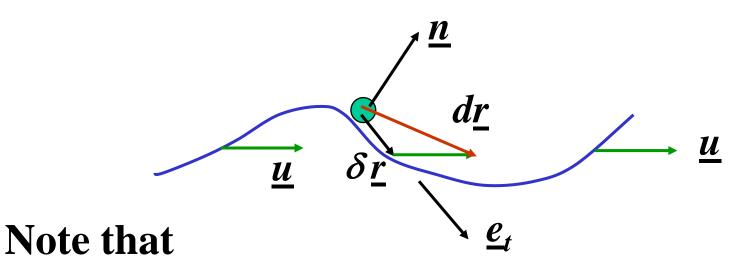
$d\underline{r}$  - is along absolute velocity direction, whereas  $\delta \underline{r}$  - is along relative velocity or tangent to the surface (frozen constraint) (set dt = 0).
