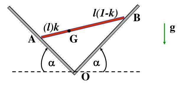
The constraints are: the ends must remain in contact with respective surfaces.
