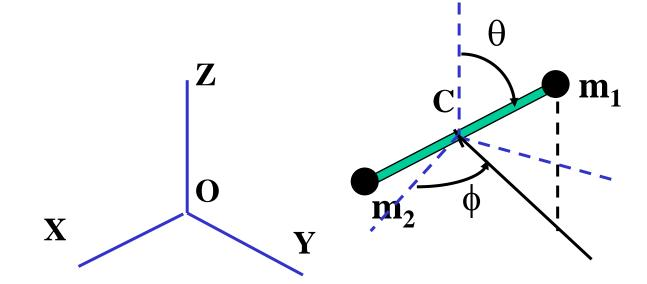
Location of center of mass  $C:(x_c, y_c, z_c)$ ; and orientation of the rod: ( $\phi$ ,  $\theta$ ). These are independent  $\rightarrow$  no constraint relation for these variables.
