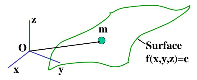
Now, the motion is confined to a prespecified surface (e.g. a roller coaster). The surface is defined by the relation:
