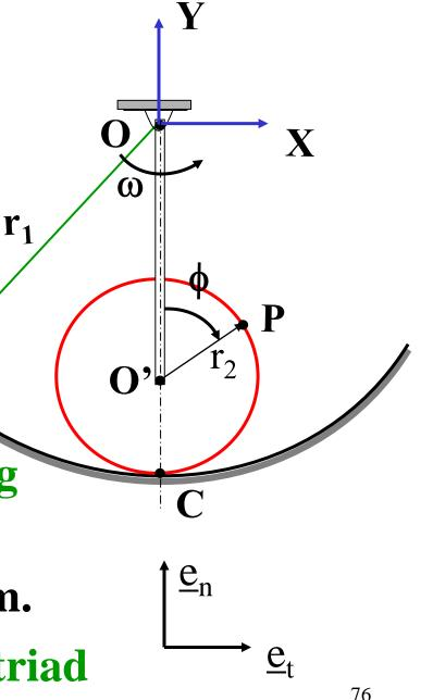
$$\underline{v}_{P} = \underline{\dot{R}} + (\underline{\dot{\rho}})_{r} + \underline{\omega} \times \underline{\rho} = \underline{v}_{O'} + (\underline{\dot{\rho}})_{r} + \underline{\omega} \times \underline{\rho}$$
