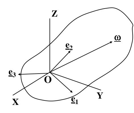
Let  $e_1, e_2, e_3$  be an independent set of unit vectors attached to a rigid body rotating with angular velocity
