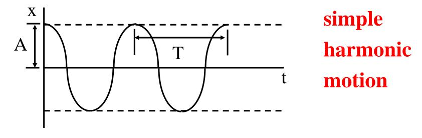
$T=2\pi/\omega$  - time period of harmonic motion  $\omega$  - circular frequency
