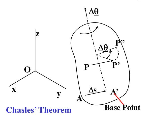
Consider displacement in time  $\Delta t$ . (displ. + rot.)Shown is an infinitesimal displacement of a rigid body
