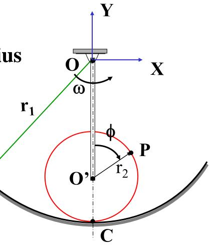
Find: The velocity  $v_p$ and acceleration  $\underline{a}_{P}$  of a point P on the wheel, specified by angle  $\phi$ w.r.t. line *00'*.
