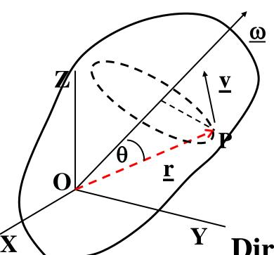
The rigid body rotates about point O (fixed base point). P - a point fixed in the body.
