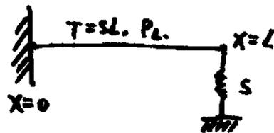
The wave equation is  $\frac{\partial^2 y}{\partial x^2} + k^2 y = 0$ .
