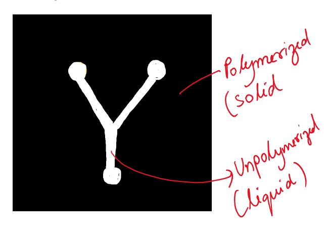
This configuration is used for design of microchannels where the surrounding is polymerized (solidified) so that a channel is obtained.
