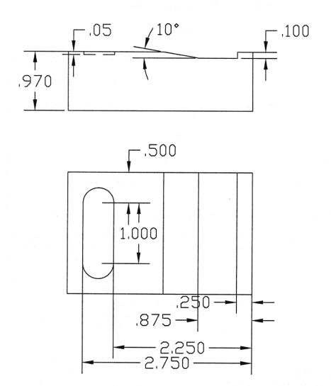
All dimensions must be within tolerance of 0.002". The angle of the slope should be within tolerance of 0.1 degrees.
