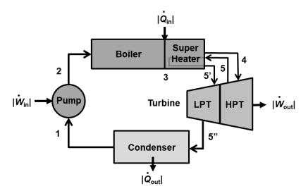
cycle in HW 34. Draw the *T-s* diagram for the reheat cycle.
